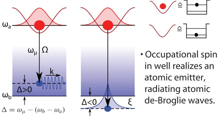
$$\hat{H}_{ab} = \sum_{\vec{k}} \frac{\hbar\Omega}{2} \gamma_{\vec{k}} e^{-i\Delta_k t} \hat{b}_{\vec{k}}^\dagger |0_a\rangle \langle 1_a| + \text{H.c.}$$
