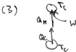
$$K = \frac{|Q_C|}{|W|} = \frac{|Q_H| \cdot \frac{T_C}{T_H}}{|W|} = \frac{100\text{J} \cdot \frac{200\text{K}}{300\text{K}}}{33.3\text{J}} = 2$$
