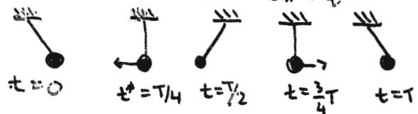
(2)  $E_{\text{kin, max}} = E_{\text{pot, max}} = mgh = mg(L - L \cos \theta)$
