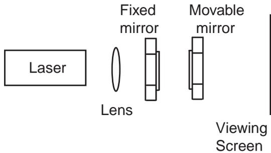
Figure 1: Schematic view of the Fabry-Perot Interferometer.
