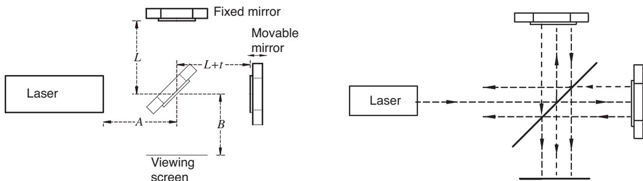
Figure 1: The Michelson interferometer. Left: equipment layout and distances. Right: ray paths. The offsets between ray paths are not real; they're just put in here for clarity.
