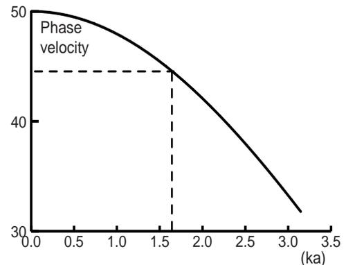
Fig. 4: This is plot of phase velocity given by  $\omega/k$ , and is taken directly from the dispersion equation, Eq. 4. It is very nearly constant at small  $k$ -values (note the vertical scale). It changes by only 10% even for  $ka/2 = \pi/4$  (dashed lines).
