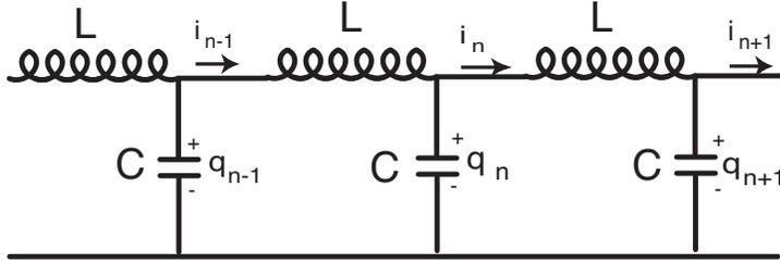
Figure 2: Schematic diagram of a three-unit LC transmission line. Because the capacitors and inductors are discrete instead of the continuous capacitance and inductance of a real transmission line, this is sometimes called a “lumped constant” transmission line. We’ll avoid the term here because it’s awkward, but you’re quite likely to see it again.
