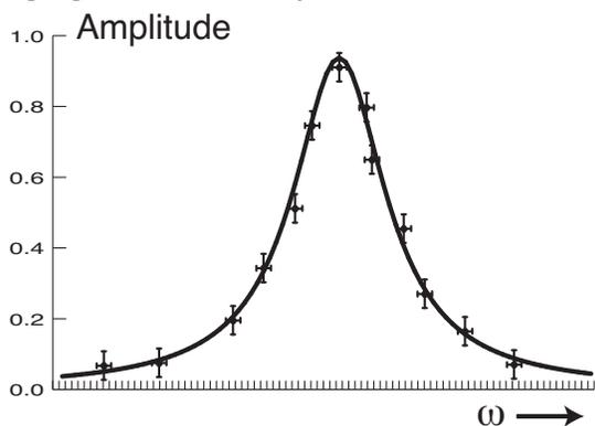
FIG. 2. The “measured” amplitudes are plotted against the driving frequency, and each data point has error bars in both dimensions. Each amplitude was measured several times, the results were averaged, and the uncertainty is the standard deviation from the average. The plotted values have all been divided by the measured maximum value. The (smaller) error bars on the frequency derive from estimates of the precision of reading the counter. The smooth curve was fitted to the data.
